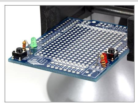
Next, we'll add the buttons to the board. They snap in place at locations BTN1 and RESET (possibly BTN2). Flip the board over, solder the leads, and trim. Easy!
